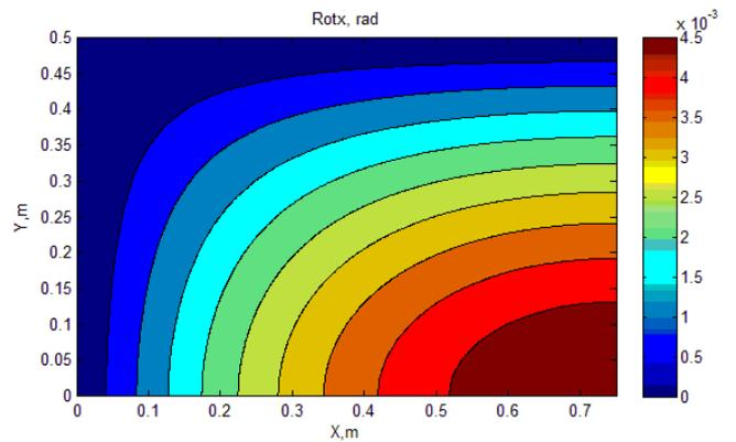
Fig. 8 Rotation around x-axis of non-optimized plate
