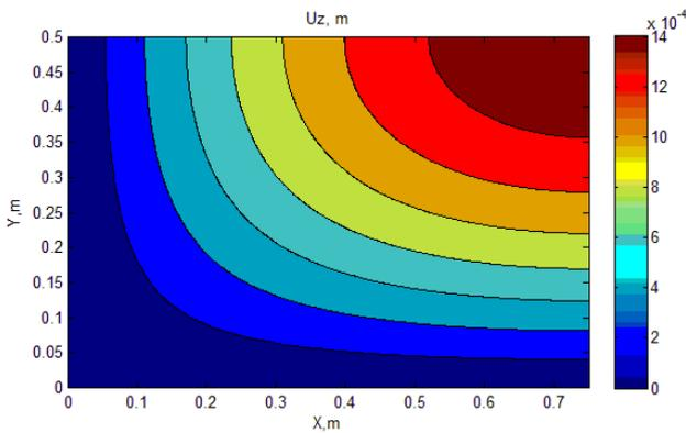
Fig. 6 Transversal displacements (m) of non-optimized plate
