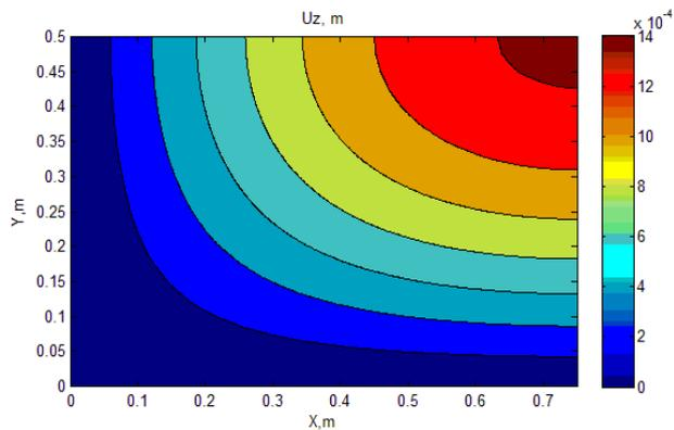
Fig. 7 Transversal displacements (m) of optimized plate
