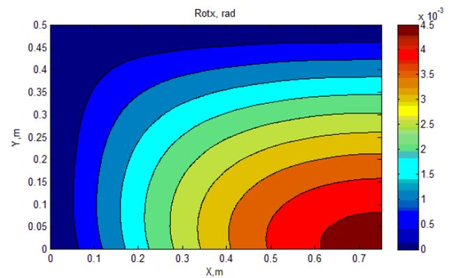
Fig. 9 Rotation around x-axis of optimized plate
