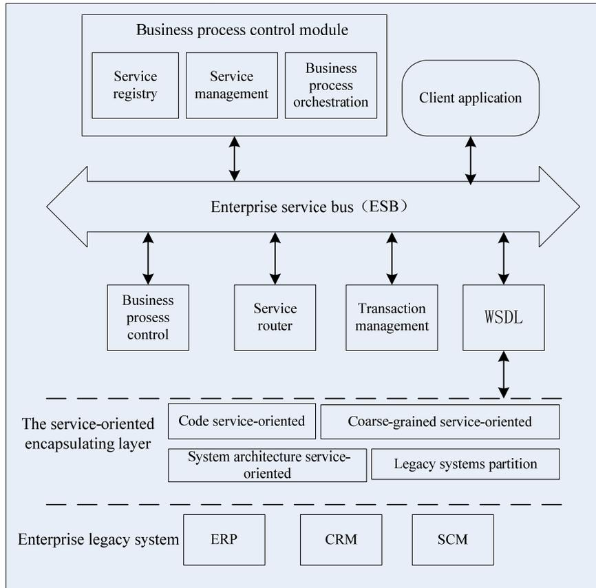
Fig. 1 The service-oriented encapsulating framework of legacy system
