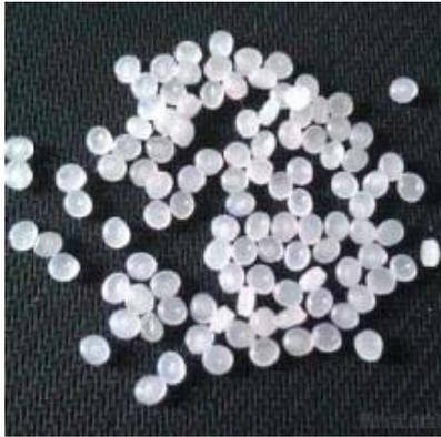
Fig. 1 Image of polypropylene (PP) granules
