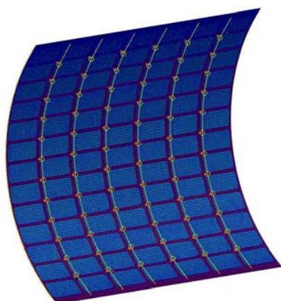
Fig. 8 Finite Element Model of Composite skin panel structure
