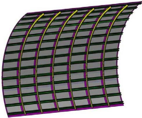
Fig. 1 CAD Model of Metallic skin panel structure
