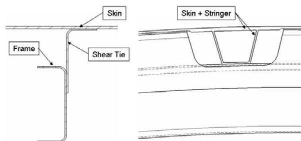
Fig. 7 Section view of composite skin panel attachments
