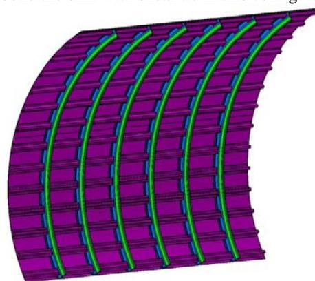
Fig. 6 CAD Model of Composite skin panel
