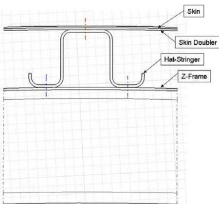
Fig. 2 Section view of metallic skin panel attachments
