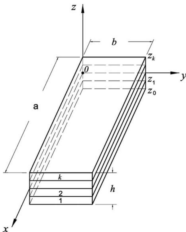
Fig. 1 The coordinate system of the composite laminated plate
