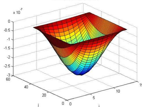
Fig. 4-a Laminated SSSS plate,  $\lambda^2 = 2.558$
