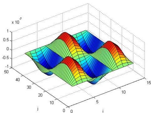
Fig. 4-h Laminated SSSS plate,  $\lambda^2 = 13.0316$
