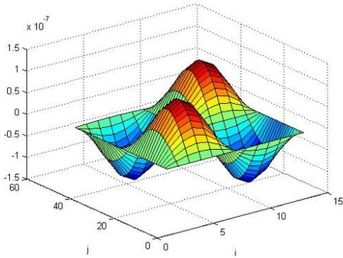
Fig. 4-e Laminated SSSS plate,  $\lambda^2 = 10.2827$
