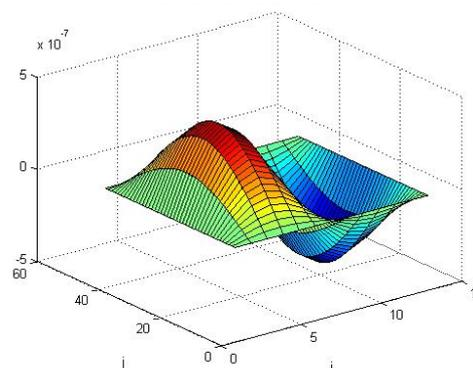
Fig. 4-d Laminated SSSS plate,  $\lambda^2 = 4.6832$
