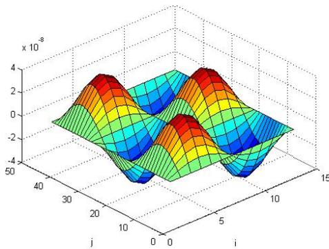
Fig. 4-f Laminated SSSS plate,  $\lambda^2 = 21.4054$
