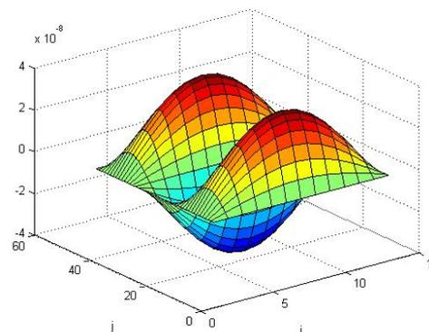
Fig. 4-c Laminated SSSS plate,  $\lambda^2 = 20.8454$
