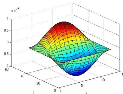
Fig. 4-b Laminated SSSS plate,  $\lambda^2 = 9.2901$
