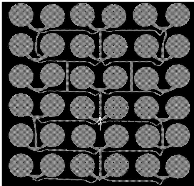
Fig. 4 36 elements circular patch microstrip array antenna
