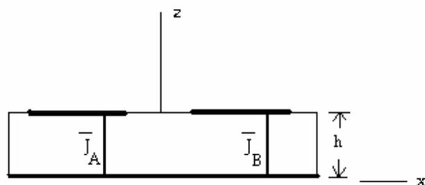
Fig. 3 Model used for mutual coupling analysis
