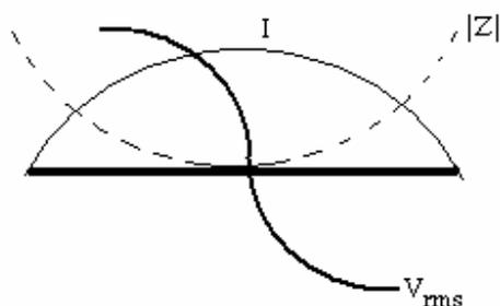
Fig. 2 Voltage, current and impedance distribution at resonant
