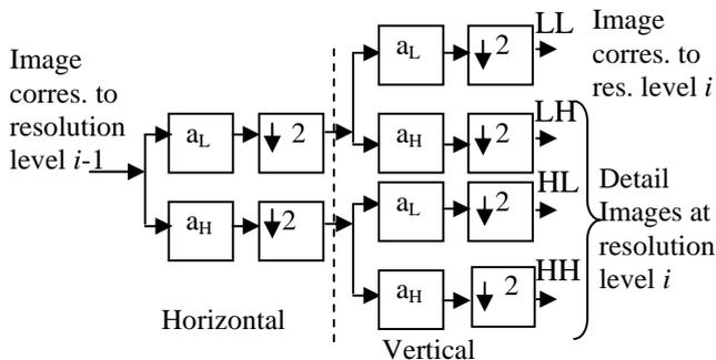
Fig. 1 One Filter Stage in 2D DWT
