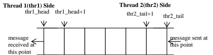
Fig. 16 Channel for reply from thread 2 to thread 1
