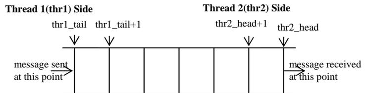
Fig. 15 Channel for message from thread 1 to thread 2
