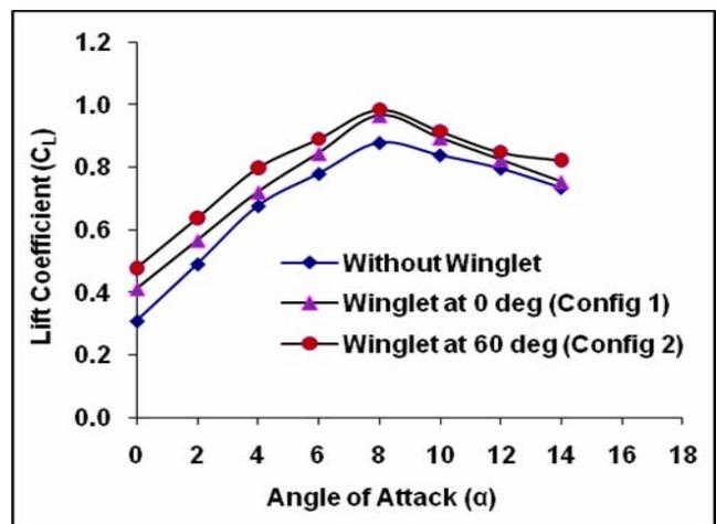
Fig.7. Lift Coefficients for the Aircraft Wing Model
