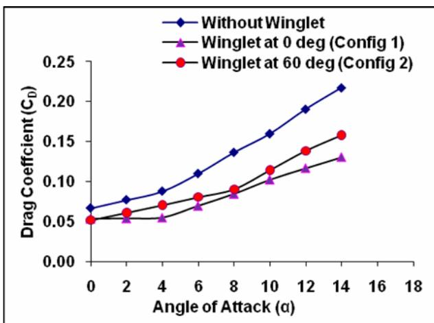
Fig.8. Drag Coefficients for the Aircraft Wing model.
