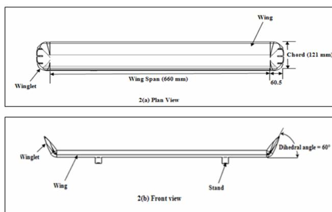
Fig. 2. Rectangular Wing with Winglet using Adapter
