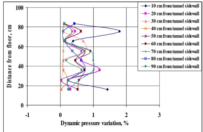
Fig.6. Dynamic pressure variation in the test section
