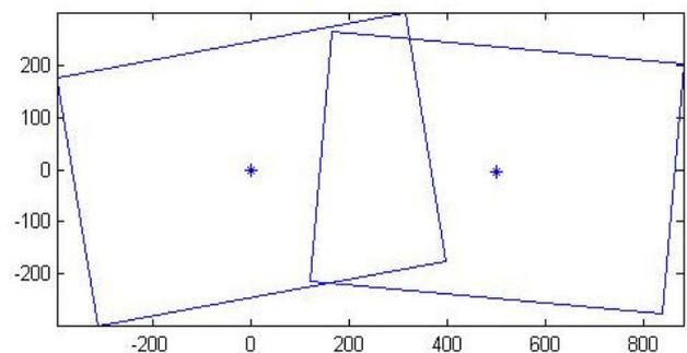
Fig. 5 Self-localization estimation result the last posture is  $(0, 0, 10^\circ)$ , the relative posture of the interest point in last image is  $(610, 40, 10^\circ)$  the relative posture of the interest point in current image is  $(50, 20, 25^\circ)$ , the current posture is  $(501.1184, -5.8075, -5^\circ)$
