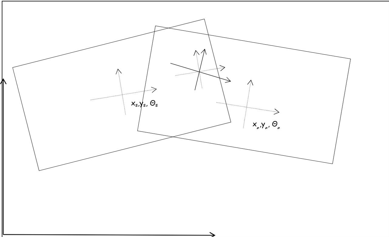
Fig. 4 Self-localization estimation method two image (two rectangles) center points represent the last posture  $X_s$  and current posture  $X_e$ . Two images contain the same interest point. The relative orientation of the interest point is different
