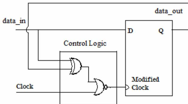
Fig. 1. Switching unit of LFSR with Modified Clock.
