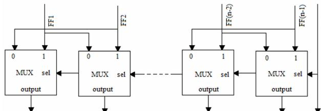
Fig. 2 Architecture of Bit Interchanging Module.
