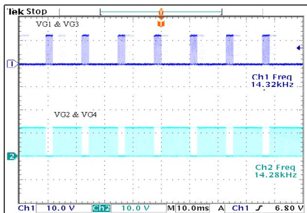
Fig. 6 Firing signal for the single phase inverter
