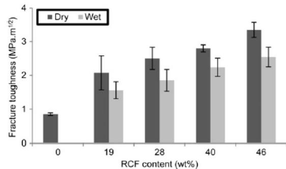
Fig. 14 Effect of fiber content on fracture toughness of dry and wet RCF/epoxy composites [7]
