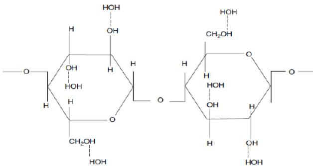
Fig. 2 Schematic of moisture absorption by natural fibre [6]
