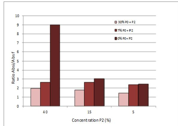
Fig. 4 Water absorption coefficient ratio (48h) between untreated recycled concrete aggregates (reference) and recycled aggregate treated versus P0 and P2 concentration by P0 and P2 applied on BO recycled concrete aggregates with 12-20mm
