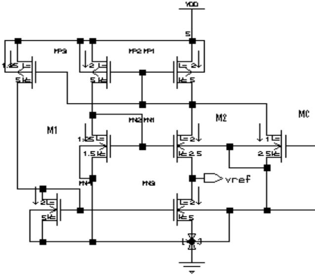
Fig. 2. CMOS PTAT temperature sensors with transistor Compensation
