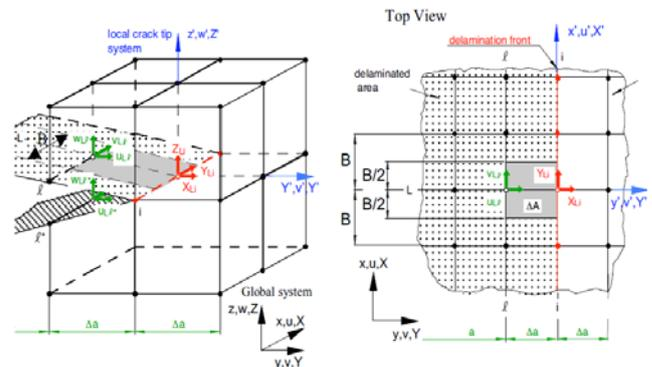
Fig. 2 Delamination front region of finite element models
