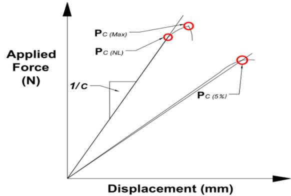
Fig. 4 Typical load-displacement responses from ECT tests
