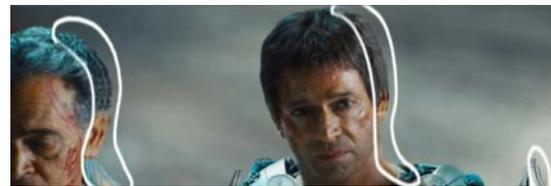
Fig. 10 An issue of double edges from right view after stereo conversion. It caused by an improperly created clean plate
