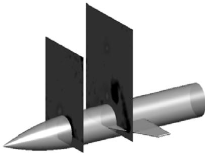
Fig. 10 Vorticity slices at  $x/D=2.5$  &  $4.35$ ,  $\gamma=30^\circ$ ,  $\alpha=45^\circ$ ,  $Re\ 0.9\ 10^5$
