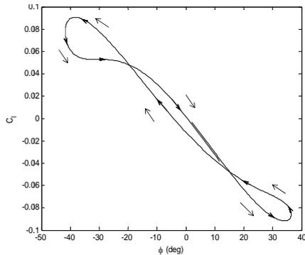
Fig. 9 Typical variation of  $C_1$  in one cycle of roll oscillation
