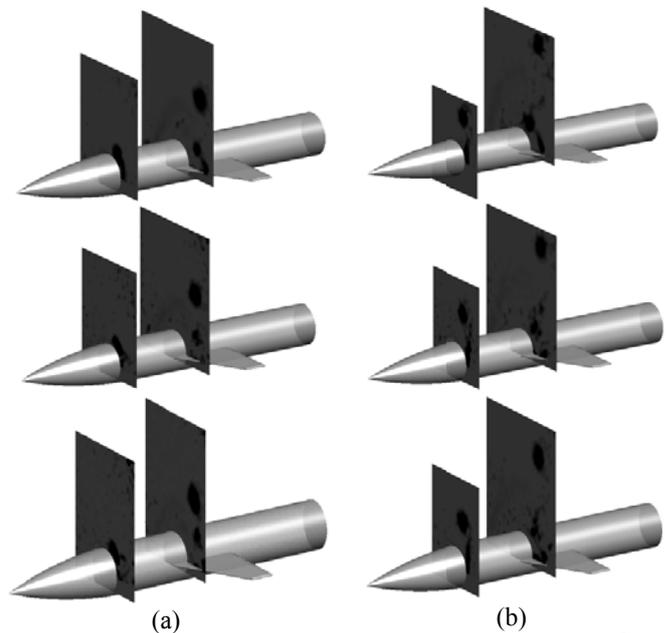
Fig. 12 Vorticity contour slices at  $x/D=2.5$  &  $4.35$ ,  $Re\ 0.9 \times 10^5$ ,  $\gamma=-30^\circ$ ,  $\phi=0^\circ$  and  $\dot{\alpha}=0$  (static),  $7.5 \times 10^{-3}$  and  $1.88 \times 10^{-2}$  [top to bottom]. a)  $\alpha=45^\circ$  b)  $\alpha=52.5^\circ$
