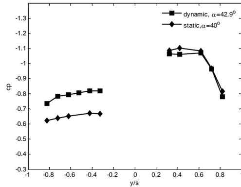
Fig. 14 Upper surface cp distributions at  $x/D = 4.85$ ,  $\gamma=45^\circ$ ,  $\bar{\omega}_p = 0$  &  $1.88 \times 10^{-2}$  at  $\alpha$  corresponding to  $max|C_l|$
