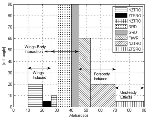
Fig. 3 Characterization of angle of attack regions based on roll motion characteristics and dominant source of asymmetry
