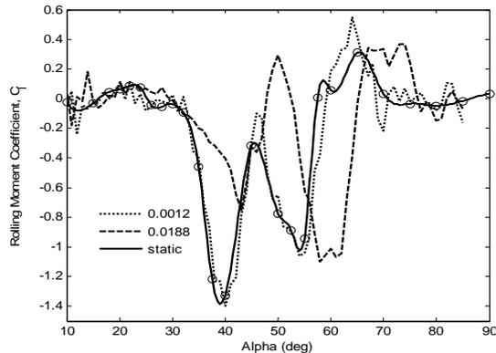
Fig. 13 Effect of pitch rate on total rolling moment coefficient,  $\gamma=45^\circ$ ,  $\varphi=0^\circ$
