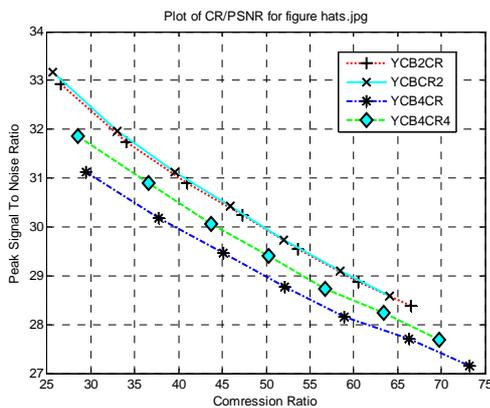
Fig. 5 Comparison of PSNR values against Compression Ratio
