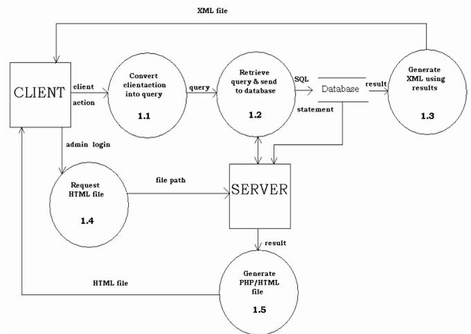
Fig. 1 Data Flow Diagram, Level 1
