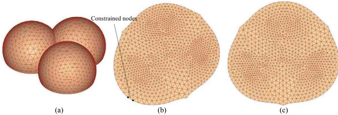
Fig. 2 Flattening of three ball surface (a) three ball model, (b) initial planar graph by intrinsic characteristic preserving, (c) flattening results by linear-elastic finite element method
