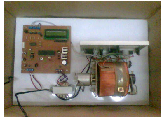
Fig. 9 A photo of constructed AVR system
