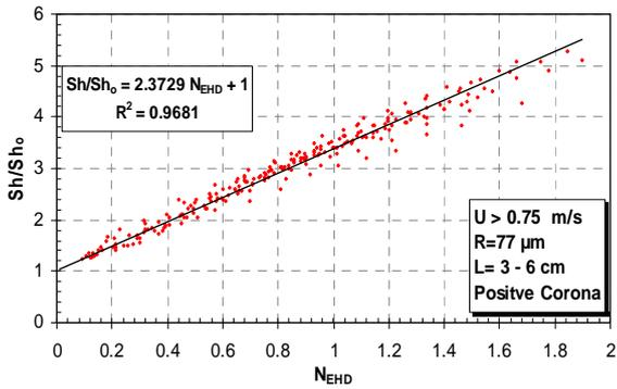
Fig. 5 Evaporation enhancement versus EHD number
