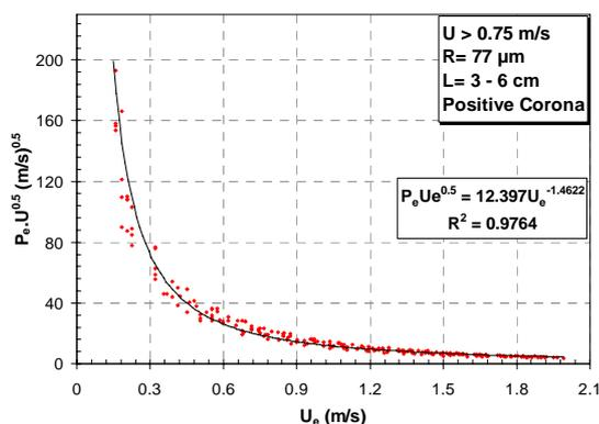
Fig. 8 EHD performance versus corona wind velocity
