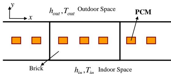
Fig. 1 Schematic view of brick with PCM
