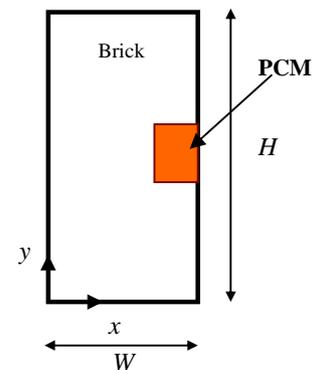
Fig. 3 Computational domain of brick with one PCM
