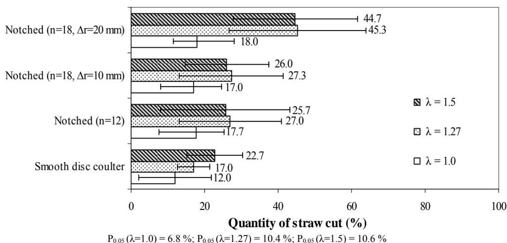
Fig. 2 Influence of the single-disc coulters form, speed ratio  $\lambda$  and straw humidity on spring barley straw cutting, humid -  $W=20.4$  %
