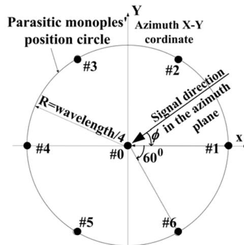
Fig. 3. Geometry of a 7-element ESPAR Antenna.
