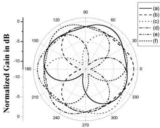
Fig. 8. Beam patterns (a) to (f) in the Azimuth Plane for Antenna Sampling Periods #1 to #6. Load Setting:  $x_1 = 0 \Omega$ ,  $x_2 = 30 \Omega$ ,  $x_3 = 0 \Omega$ ,  $x_4 = 30 \Omega$ ,  $x_5 = 30 \Omega$ ,  $x_6 = 30 \Omega$ .
