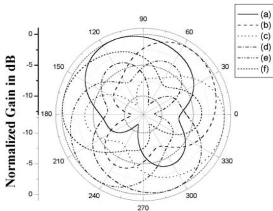
Fig. 10. Beam Patterns (a) to (f) in the Azimuth Plane for Antenna Sampling Periods #1 to #6. Load Reactance:  $x_1 = 0 \Omega$ ,  $x_2 = 10 \Omega$ ,  $x_3 = 0 \Omega$ ,  $x_4 = -30 \Omega$ ,  $x_5 = 70 \Omega$ ,  $x_6 = 30 \Omega$ .
