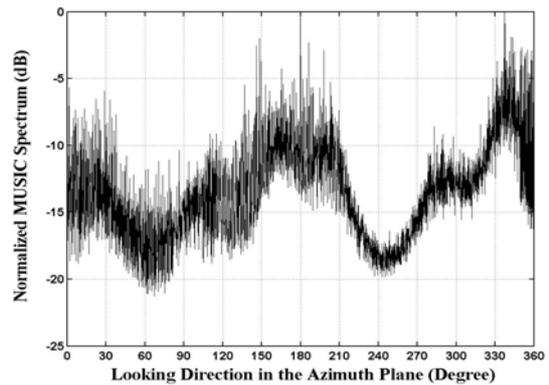
Fig. 7. MUSIC Spectrum for Case 2:  $x_1 = 0 \Omega$ ,  $x_2 = 30 \Omega$ ,  $x_3 = 0 \Omega$ ,  $x_4 = 30 \Omega$ ,  $x_5 = 0 \Omega$ ,  $x_6 = 30 \Omega$ . SNR = 40 dB. Signal Directions: 120°, 150° and 300° in the Azimuth Plane.
