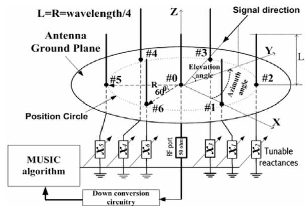
Fig. 2. Configuration of a 7-element ESPAR Antenna [6].
