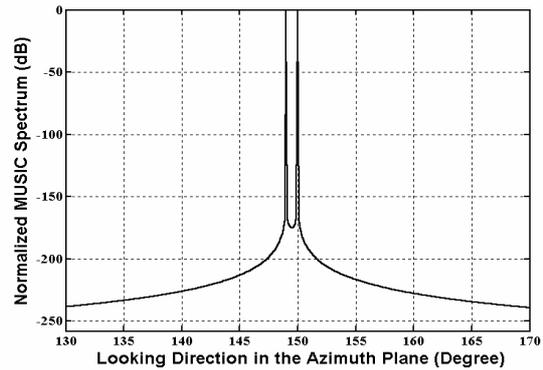
Fig. 13. MUSIC spectrum. Load Setting is Same as for Case 3. SNR=30 dB. Two Signal Directions Are 149°, and 150°, respectively, in the azimuth plane.
