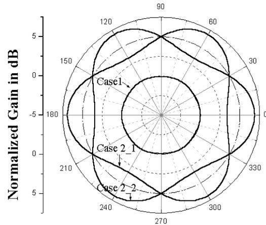
Fig. 5 Beam Pattern for Case 1 (Equal load reactance of 30 $\Omega$ ) and Two Possible Beam Patterns in Case 2 ( $x_1 = 0 \Omega$ ,  $x_2 = 30 \Omega$ ,  $x_3 = 0 \Omega$ ,  $x_4 = 30 \Omega$ ,  $x_5 = 0 \Omega$ ,  $x_6 = 30 \Omega$ ) are shown with dot lines (Case2\_1 & Case2\_2).
