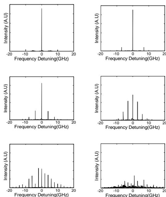
Fig. 1 Power spectra of the SL under the injection of two MLs at  $K_{1,2} = -35$  dB and  $\Delta f_{1,2}$ : (a)  $\pm 10$  GHz, (b)  $\pm 7$  GHz, (c)  $\pm 4$  GHz, (d)  $\pm 3$  GHz, (e)  $\pm 2$  GHz, (f)  $\pm 1$  GHz
