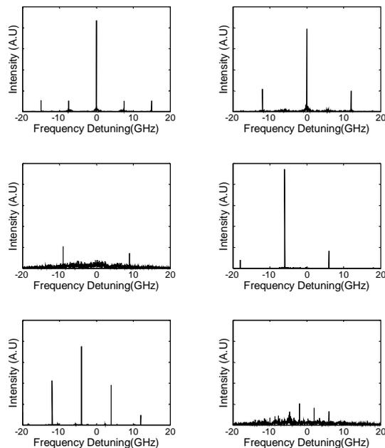
Fig. 2 Power spectra of the SL under the injection of two MLs at  $K_{1,2} = -25$  dB and  $\Delta f_{1,2}$ : (a)  $\pm 15$  GHz, (b)  $\pm 12$  GHz, (c)  $\pm 9$  GHz, (d)  $\pm 6$  GHz, (e)  $\pm 4$  GHz, (f)  $\pm 2$  GHz.
