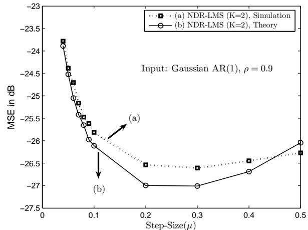
Fig. 2. Steady-state MSE of normalized data-reusing LMS (NDR-LMS) algorithm as a function of the step-size with  $K = 2$  in nonstationary environment for colored Gaussian input (Input: Gaussian AR(1),  $\rho = 0.9$ ).
