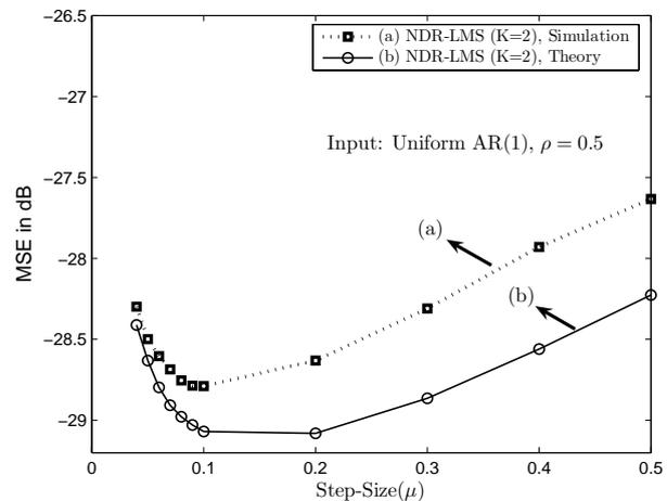
Fig. 3. Steady-state MSE of normalized data-reusing LMS (NDR-LMS) algorithm as a function of the step-size with  $K = 2$  in nonstationary environment for colored Uniform input (Input: Uniform AR(1),  $\rho = 0.5$ ).
