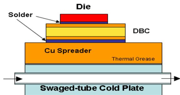
Fig. 3 Schematic of IGBT with thermal management
