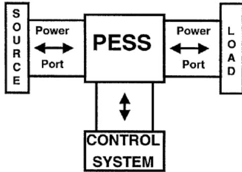
Fig. 1 Three-Port Power Electronic System Structure schema
