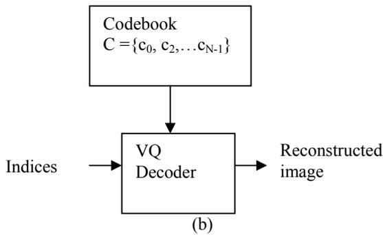
Fig. 1 (a) VQ Encoder (b) VQ Decoder
