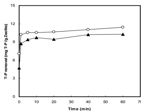
Fig. 1 Livestock wastewater treatment efficiency by zeolite adsorption (25 g zeolite/l) and electron beam irradiation (20kGy), (a)  $\text{NH}_4^+\text{-N}$  (b) T-N and (c) T-P removal,  $\blacktriangle$ , zeolite adsorption only;  $\circ$ , zeolite adsorption and electron beam irradiation
