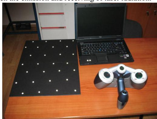
Fig. 2 3D scan system *EXA Scan 30144*
