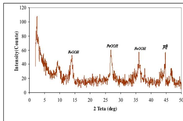
Fig. 2 X-Ray diffraction analysis of synthesized nZVI
