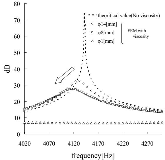
Fig. 3 Comparison of the results of the theoretical calculation and the FEM simulation for different tube diameters
