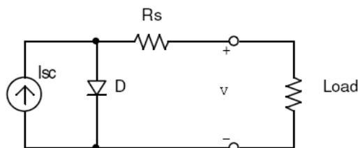
Fig. 2 Equivalent circuit of the solar cell
