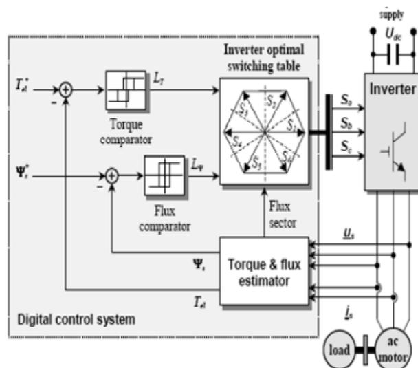
Fig. 7 Basic DTC scheme for ac motor drives
