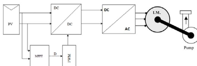
Fig. 1 Structure of the photovoltaic pumping system
