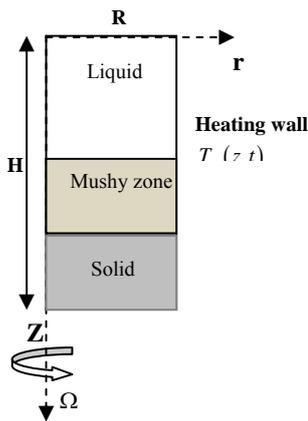
Fig. 1 Schematic of vertical Bridgman Growth (VG)
