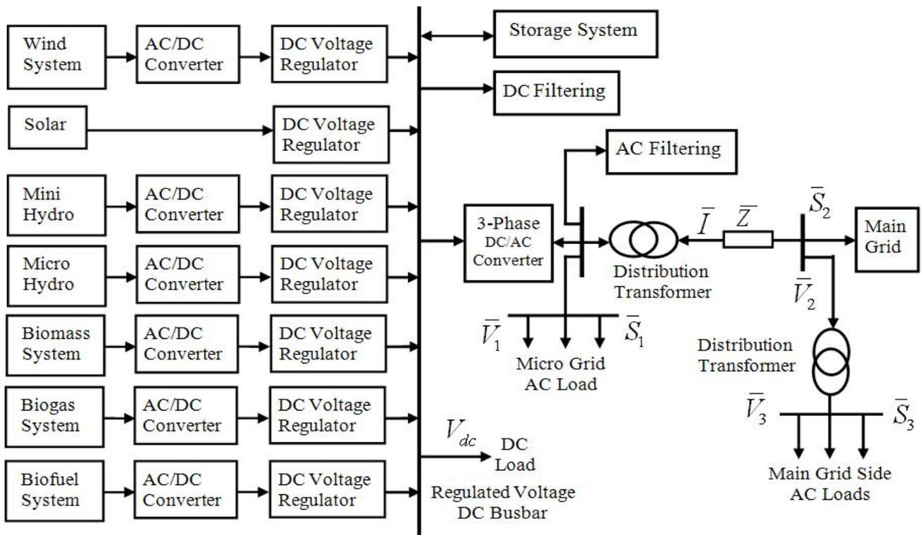
Fig. 1 Configuration of the multisource microgrid [8]
