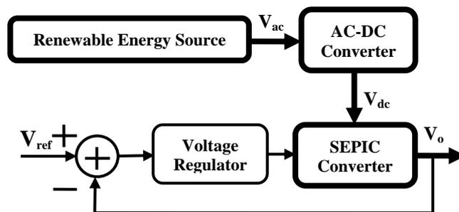
Fig. 3 DC voltage regulator based on SEPIC converter
