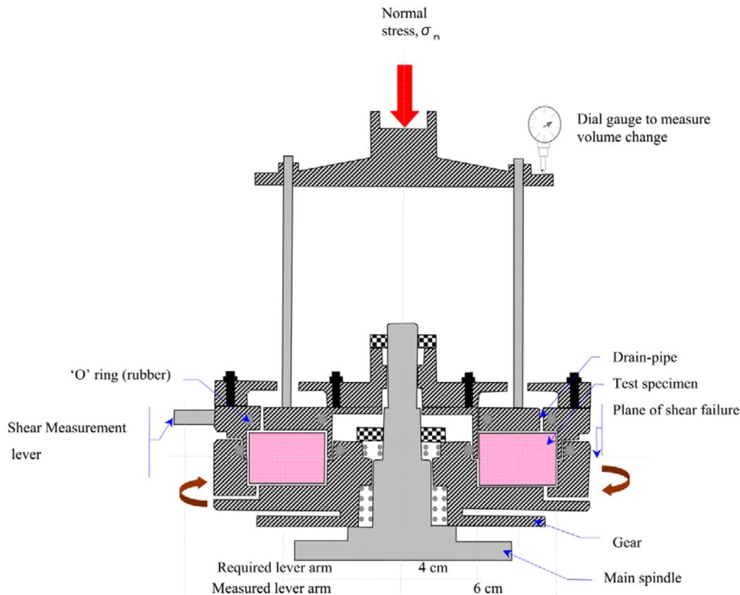
Fig. 1 Structural features of torsional ring shear apparatus
