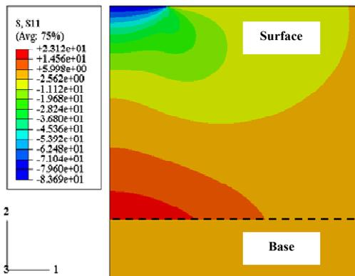
Fig. 5 Variations of horizontal stress with depth
