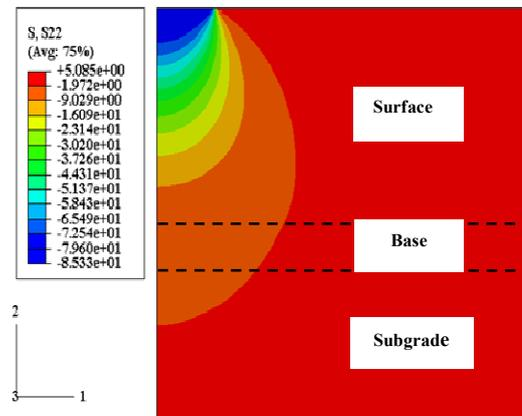
Fig. 4 Contour of vertical stress
