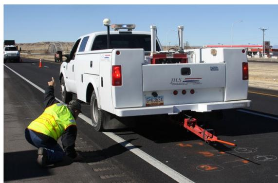
Fig. 1 Execution of FWD test
