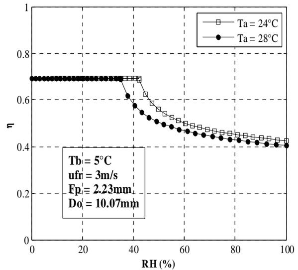
Fig. 7 Effect of air temperature on fin efficiency
