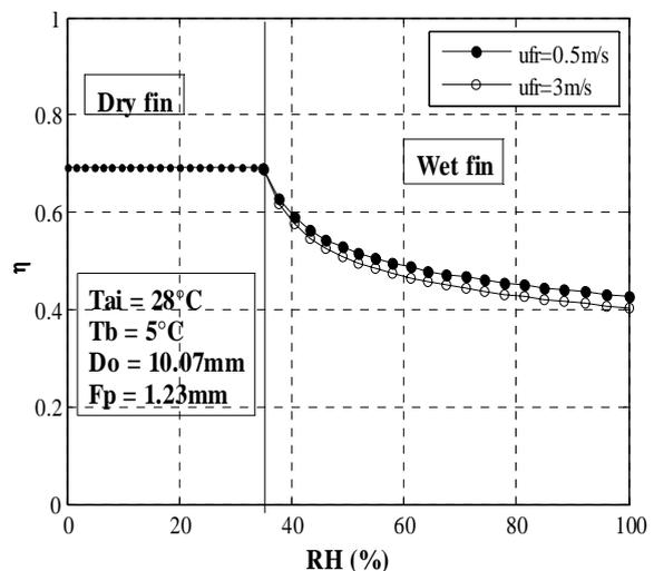
Fig. 4 Effect of frontal velocity on fin efficiency
