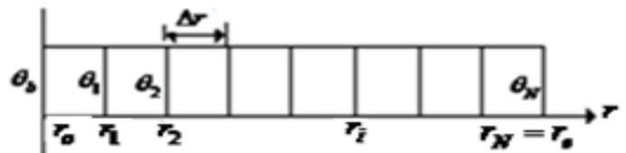
Fig. 2 Finite difference scheme for 1-D circular fin
