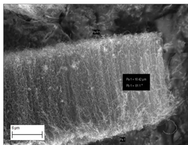
Fig. 2 Side angle view of MWCNTs scraped off substrate surface
