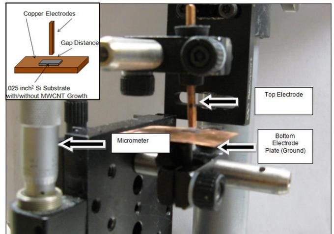
Fig. 4 Copper electrodes and micrometer stage
