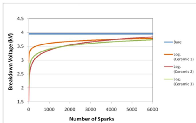
Fig. 11 Durability of MWCNT/ceramic mix over 6000 sparks
