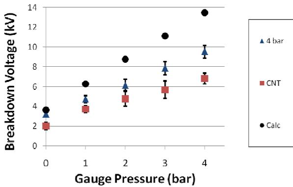
Fig. 8 Breakdown voltage vs. gauge pressure (1mm gap)
