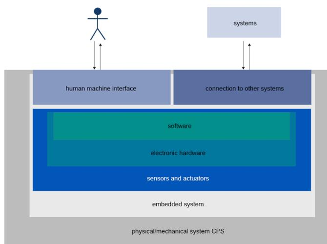
Fig. 1 Interaction between humans and machines via Cyber-Physical-Systems [11]
