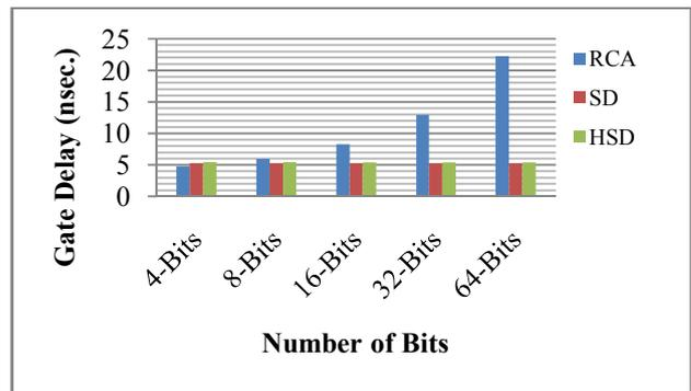
Fig. 6 (a) Gate Delay of fast adders
