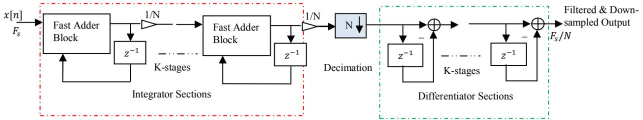
Fig. 3 Block level structure of CIC decimation filter
