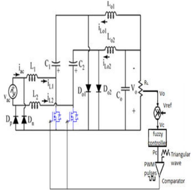
Fig. 2 Proposed circuit using Fuzzy Controller
