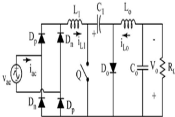
Fig. 1 Conventional Cuk PFC converter
