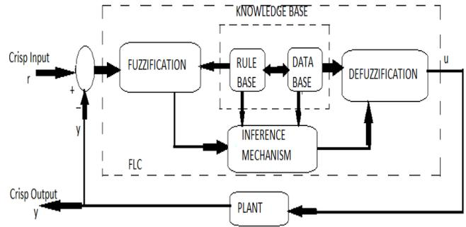
Fig. 6 Basic structure of fuzzy logic system
