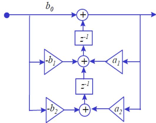
Fig. 1 Realization of a second order IIR filter
