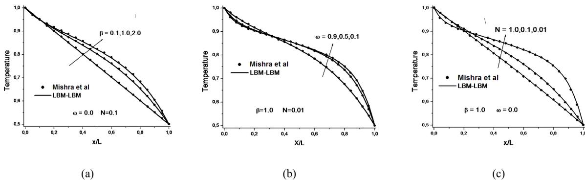
Fig. 1 Comparison of non dimensional temperature in a planar medium at the steady-state for the effects of (a) extinction coefficient, (b) scattering albedo and (c) conduction-radiation parameter
