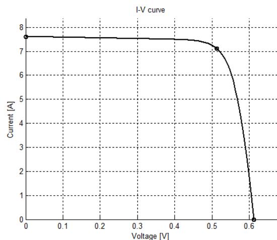
Fig. 3 VI characteristics of solar cell
