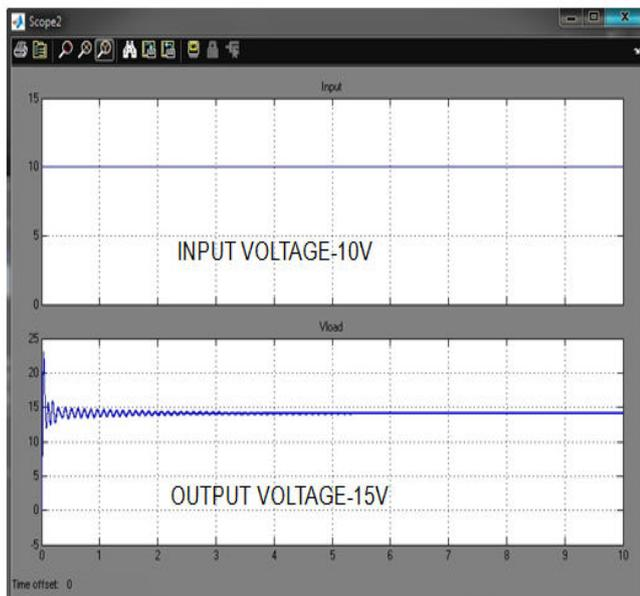
Fig. 10 Simulation Result of SEPIC Converter
