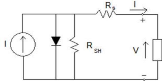
Fig. 2 Single diode model of PV cell
