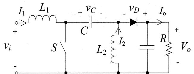
Fig. 6 Circuit diagram of a SEPIC converter
