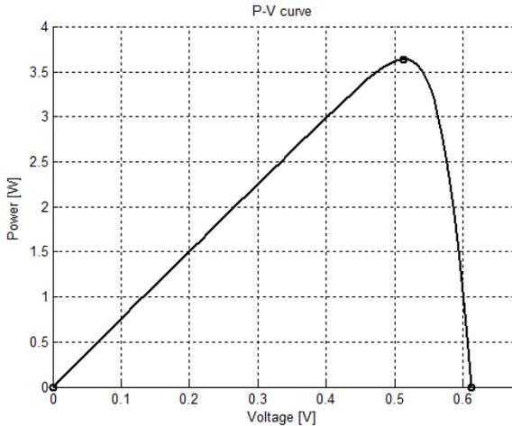
Fig. 4 P-V characteristics of solar cell
