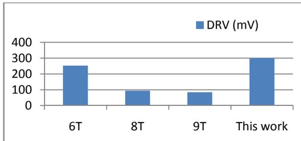
Fig. 8 Data Retention Voltage of different SRAM Cells
