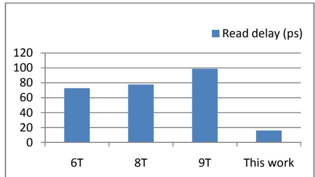
Fig. 6 Read Delay in different SRAM Cells
