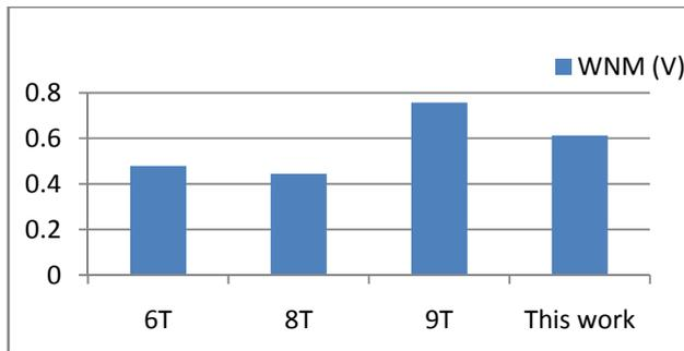
Fig. 4 Write Noise Margin in different SRAM Cells
