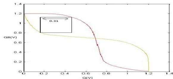
Fig. 3 Butterfly Curve for Read Noise Margin. The side of the maximum sized square indicated the noise margin as 0.31V
