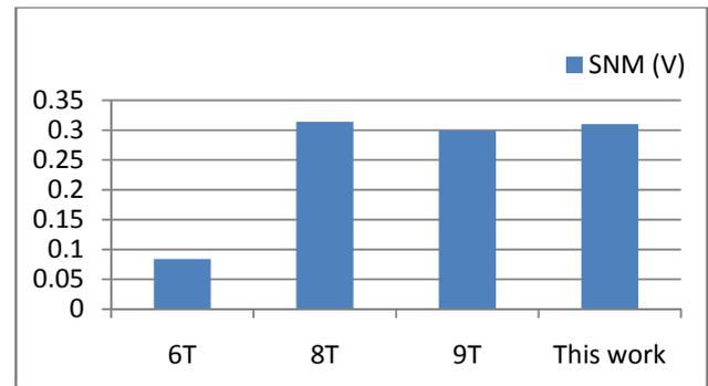
Fig. 2 Read Noise Margin in different SRAM Cells
