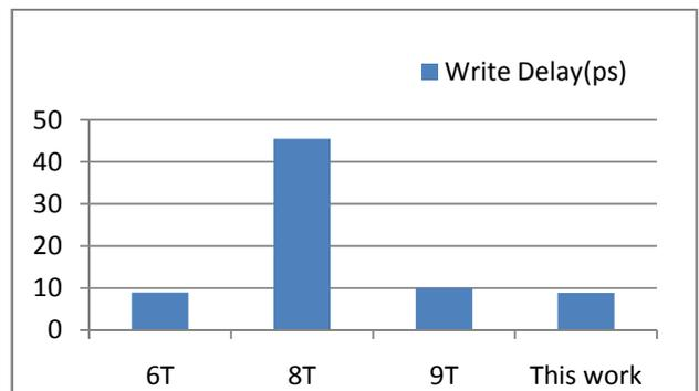
Fig. 7 Write Delay in different SRAM Cells
