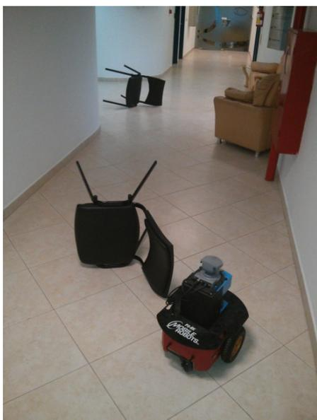
Fig. 9 Robot Pioneer 3-dx avoiding an unknown obstacle
