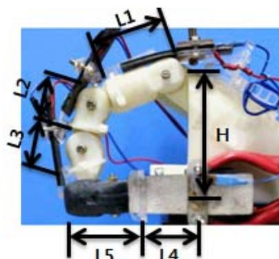
Fig. 1 An index and thumb finger dummy equipped with an exoskeleton
