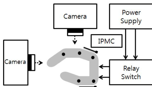
Fig. 2 Experimental setup for pinching motion analysis
