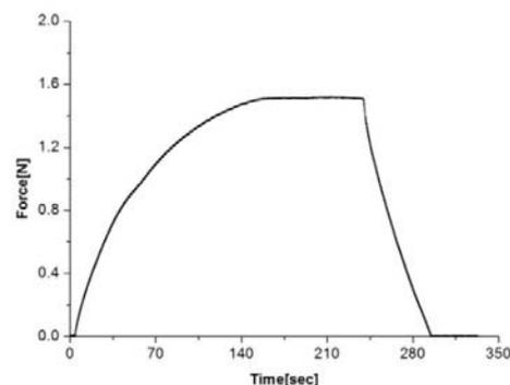
Fig. 3 Blocking force of an IPMC actuator
