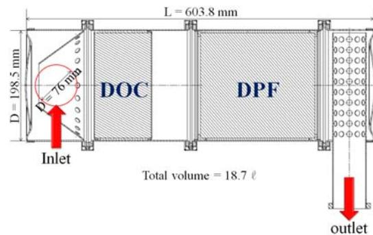
Fig. 1 Catalytic muffler adopted in this work
