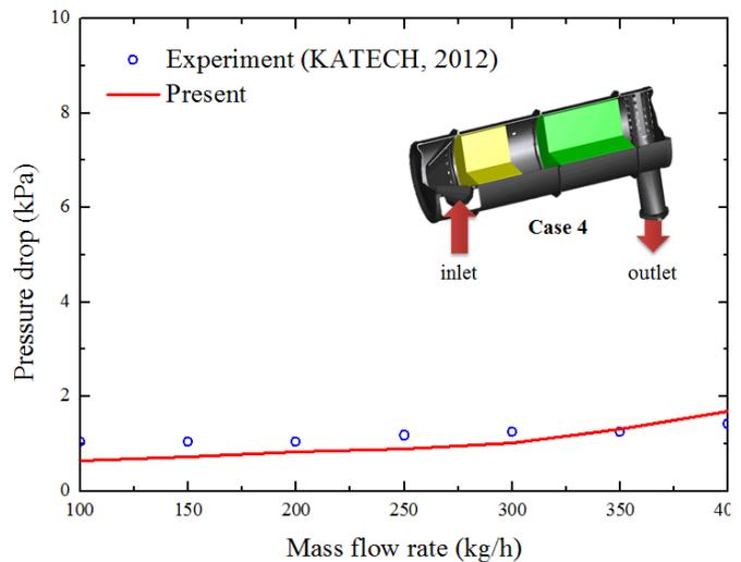
Fig. 3 Comparison of the pressure drop for the Case 4 with mass flow rate
