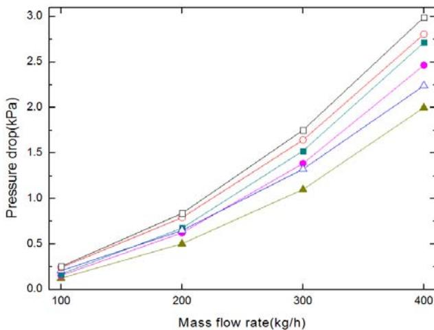
Fig. 7 Comparison of the pressure drop for the catalytic muffler with different configurations and different mass flow rates
