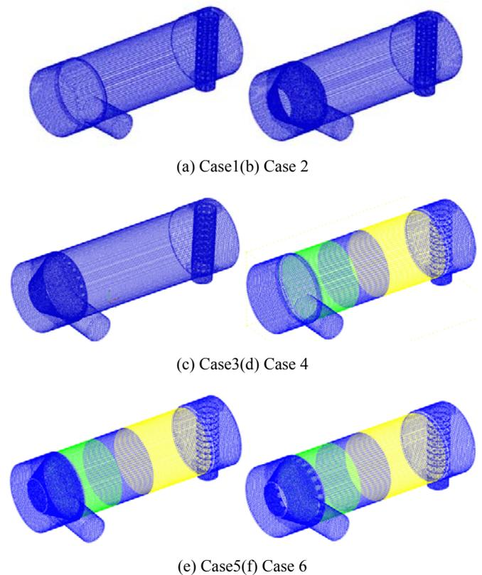
Fig. 2 Computational grid system of the catalytic muffler
